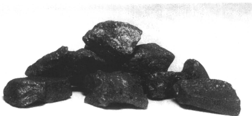
Figure 3. Ammonia synthesis catalyst
